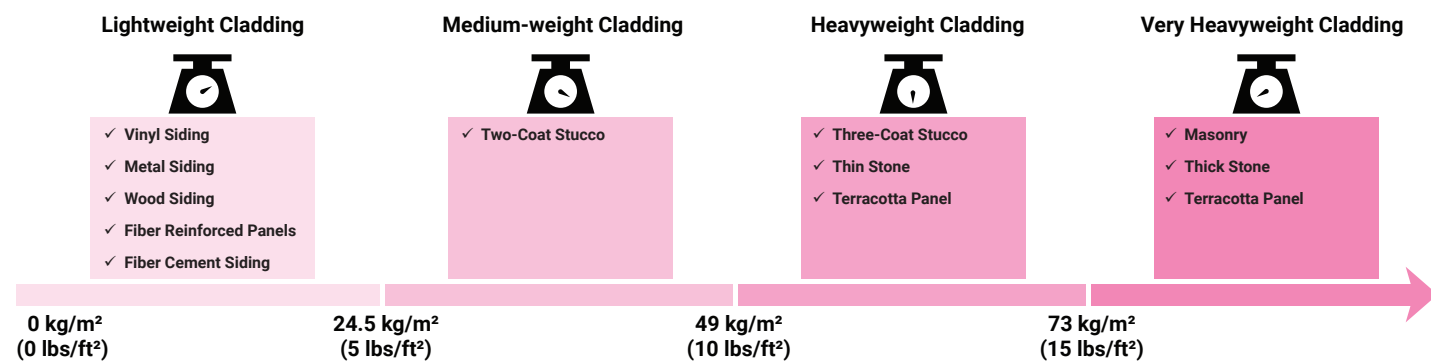
Figure 3. Cladding weight classifications. Example cladding types are listed for each classification; use the project-specific cladding weight to determine the weight classification for each cladding type.
