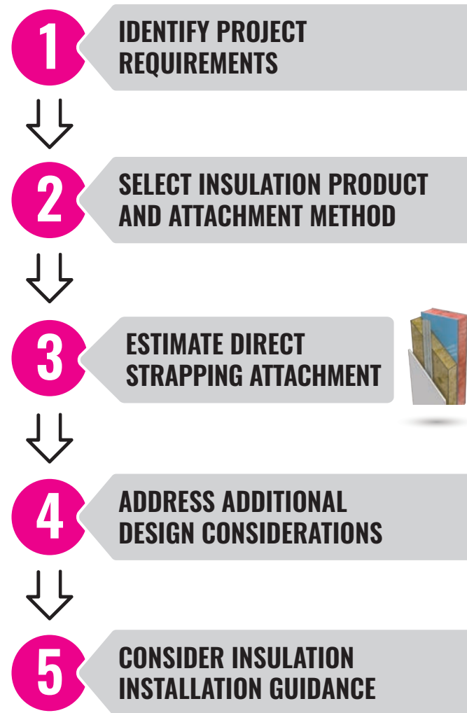
Figure 2. Steps in the continuous insulation design path.
